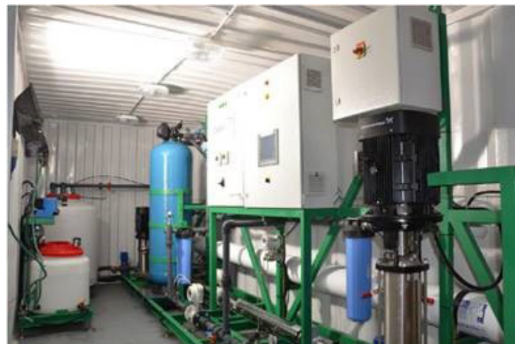
Desalitech Pilot Closed Circuit Desalination System and Conceptual sketch of a typical CCD system
